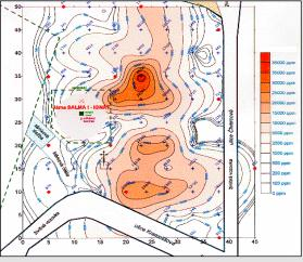
Samples of contour maps showing high Methane concentrations; the large sites surrounding closed mines were measured using GPS data logging systems.
